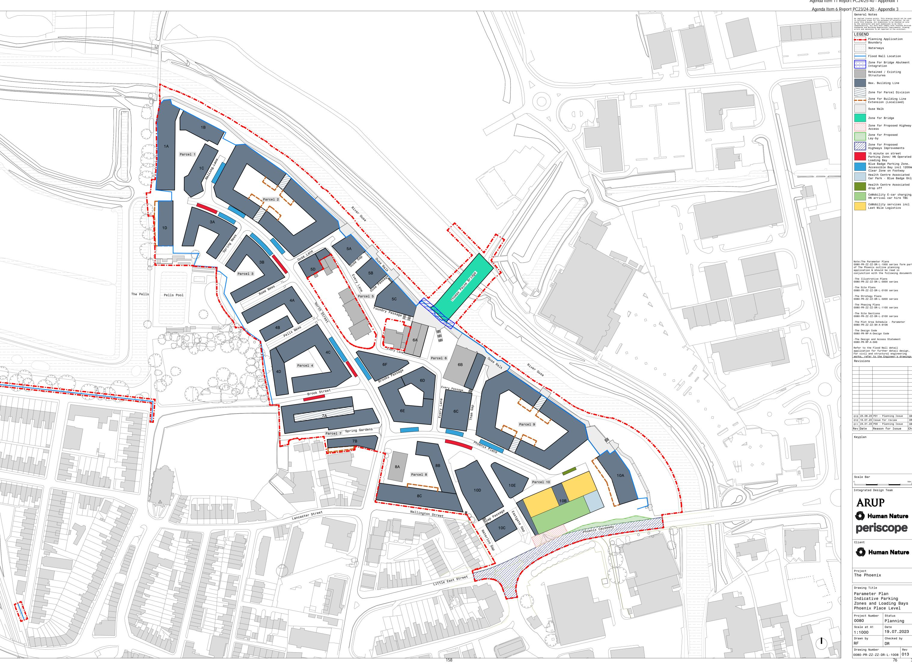
Planning Application Boundary Waterways Flood Wall Location Zone For Bridge Abutment
