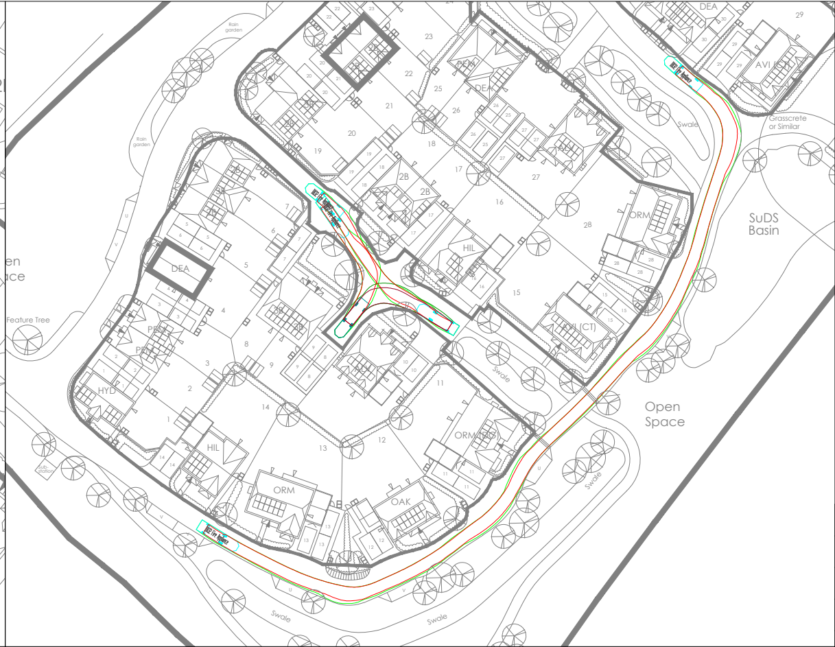
EMERGENCY VEHICLE TRACKING TURNING HEAD AND SOUTHERN SECTION (SCALE – 1:1000)
