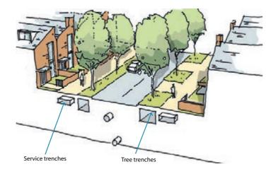
Figure 8.18: Service trenches should be designed to avoid tree planting trenches (from Architecture PLP).
