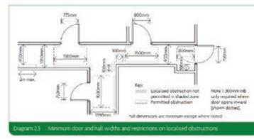
Figure 14.6: Extract from Part M for Category 2 internal dimensions.
