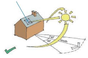
Figure 1.3: Solar collection can affect orientation of buildings or roof form.
