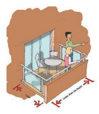
Figure 10.6: Potential dimensions for balconies.
