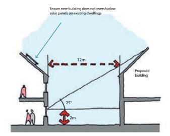
Figure 10.8: Daylighting diagram for new development adjacent to an existing property.
