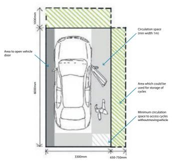
Figure 8.7: Minimum dimensions for garages (or car barns) storing bicycles (from Cambridge Cycle Parking Guide for Residential Developments).
