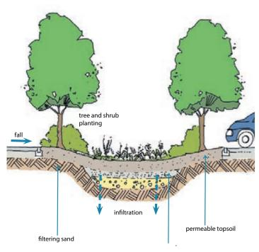
Figure 9.22: Bioretention area (from Susdrain).
