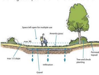
Figure 9.23: Infiltration basin (Susdrain) RELABEL.
