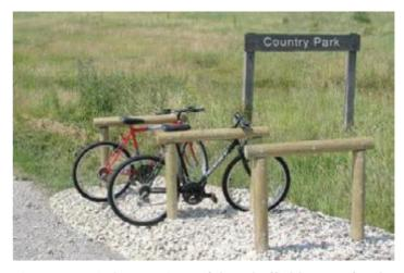
Figure 8.9: Timber versions of the 'Sheffield' type of cycle rack.
