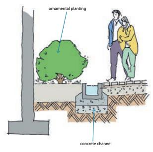
Figure 9.20: Rill with planting (from Susdrain).
