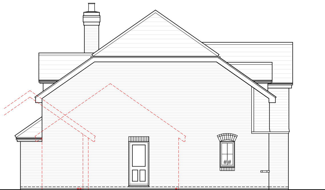
*Plot 10 - Position of Garage roof. ## No side window to Plot 10 **Plot 27 - Position of Carport roof. Refer to Site Layout & drawings for details. Side Elevation
