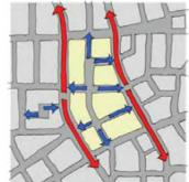
Figure 1.1: Poorly connected (a) and well connected (b) new street layout (red arrows for vehicular and blue for non-motorised traffic).
