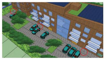
Figure 8.27: Illustration of how EV charge points could be located for flats (ringed in red).
