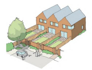
Figure 11.3: Rear gardens backing onto car parks, where unavoidable, should be in brick or stone with planting where possible
