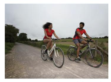
Figure 12.42: Centurion Way between Chichester and West Dean is a good example of a rural cycle (and pedestrian) route with a very simple construction using local materials. (A self-binding limestone dust over a 'Type 1' graded stone sub-base with no edge details or kerbs).
