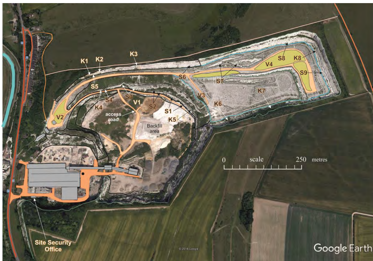
Figure 3. Plan of Upper Beeding Quarry, Shoreham Cement Works superimposed on a Google Earth image and showing localities referenced in Table 1. V=viewing point S=field section K=karst feature.
