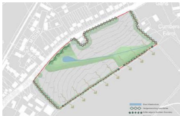
Fig 3: Layout of public open space, sustainable drainage systems and developable area respond to contours
