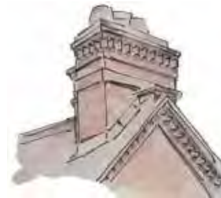
Cogging to gable end and chimney
