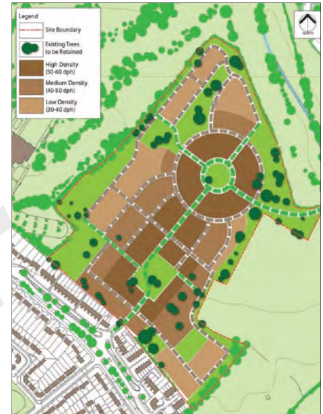
An example of a sketch design (or block) plan (Exeter Design Guide) Fig.8
