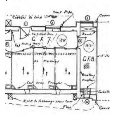
8.5 The existing masonry walls of the entrance turret and the stable wing running to the side are clearly evident on the drawing. An inward opening door aperture and a window to the space are evident to the courtyard side. This window is one of the high-set Diocletian windows, shown (though slightly obstructed by the lower scaffold) during construction in the photograph, below.
