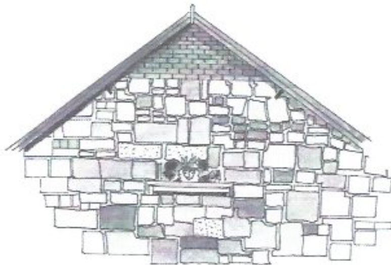
Random rubble masonry forming the gable end to the former village shop.
