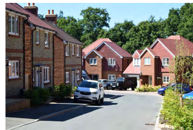
The Bailey Road development successfully uses vernacular materials; red brick, clay tiles and flint.
