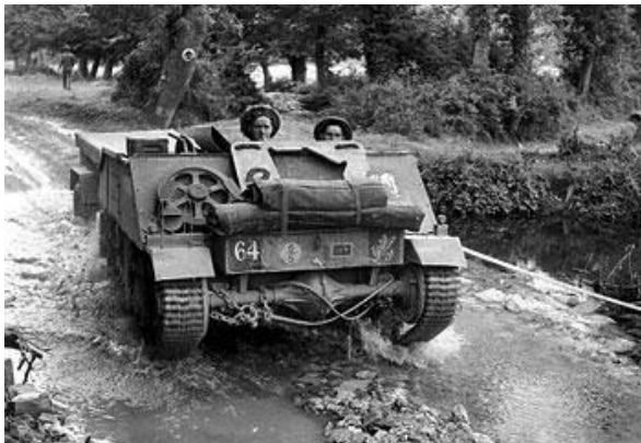
A typical Universal Carrier
