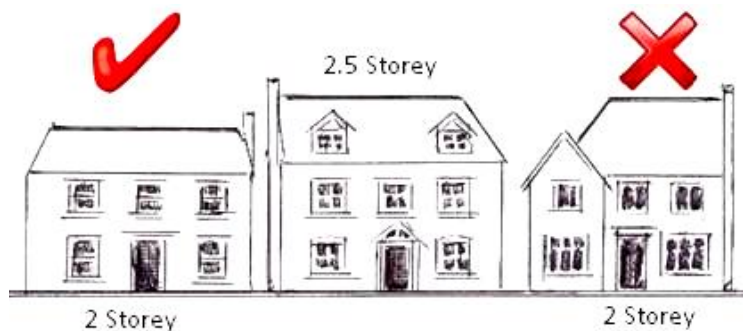
Fig 6.5: Example of Acceptable and unacceptable 2 storey heights
