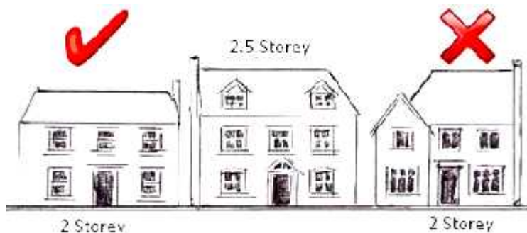
Fig 6.5: Example of Acceptable and unacceptable 2 storey heights
