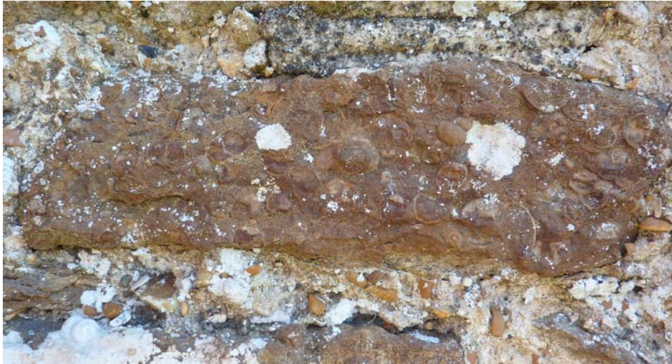
Figure 11: “Winklestone” used in the construction of the church
